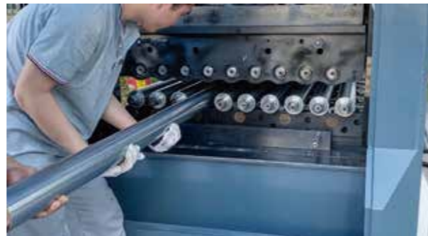
快速换滚装置 Quick roll change device
